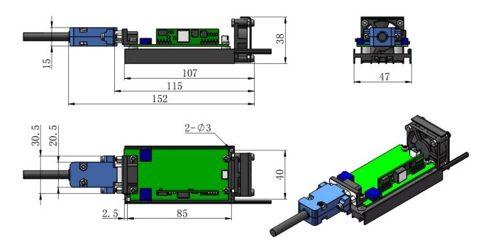
Dimensions of PSU-V-OEM and PSU-I-OEM power supply with dust cover(110×70×47mm³)
